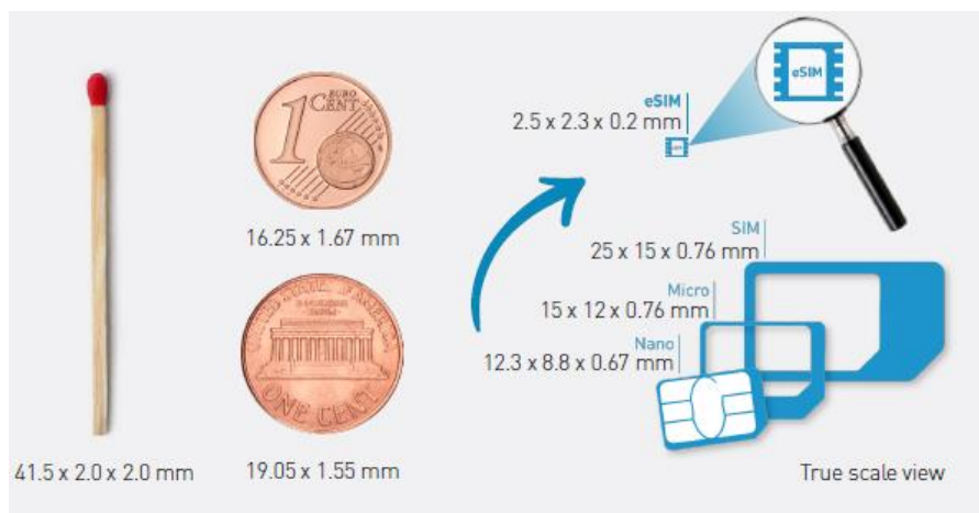
Figure 1: Showing the size of eSIM (2.5 x 2.3 x 0.2mm) [31]
